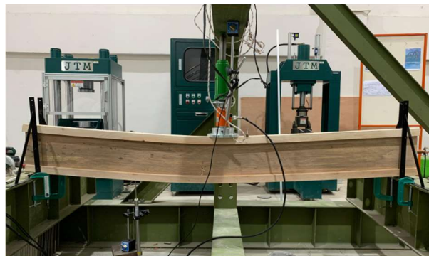
Gambar 5. Uji kuat lentur I-Joist
