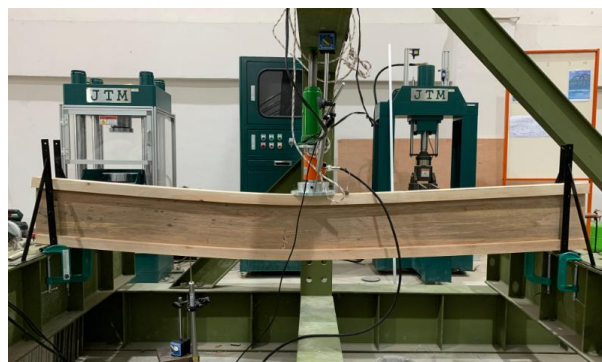
Gambar 5. Uji kuat lentur I-Joist
